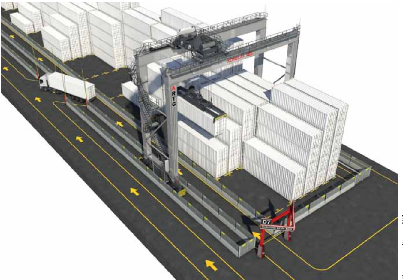
Figure 5: ARTG block layout example, brownfield layout derived from typical RTG block layout. Exchange area of one truck lane and truck by-pass lane between the blocks
